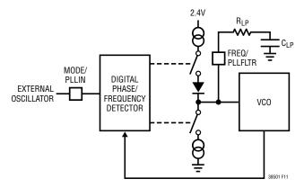
Figure 11. Phase-Locked Loop Block Diagram
