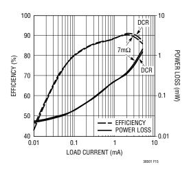
Figure 15. Design Example Efficiency vs Load
