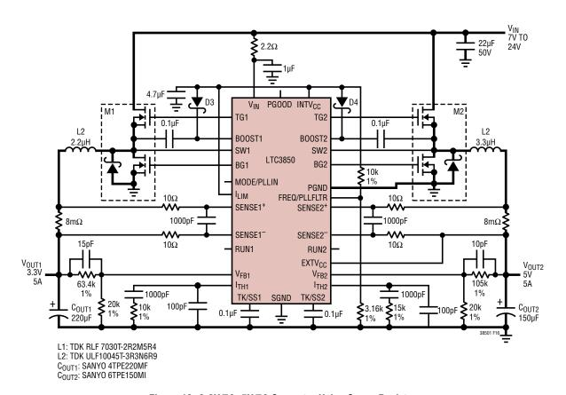
Figure 16. 3.3V/5A, 5V/5A Converter Using Sense Resistors
