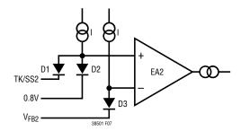
Figure 7. Equivalent Input Circuit of Error Amplifier
