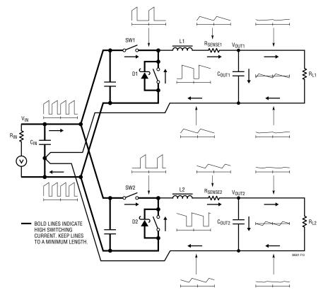
Figure 12. Branch Current Waveforms
