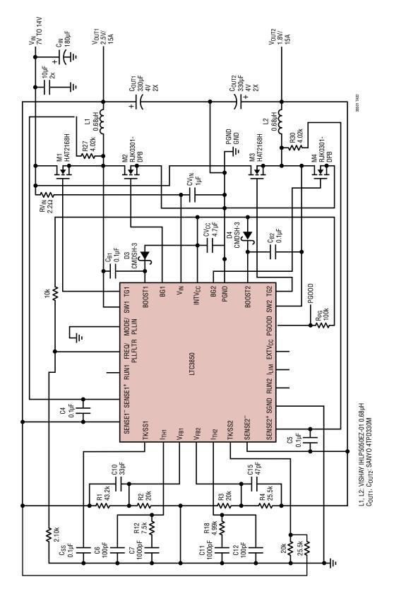
Figure 17. 2.5V/15A, 1.8V/15A Converter with DCR Sensing and Coincident Rail Tracking  $F_{SW} = 350 \text{kHz}$
