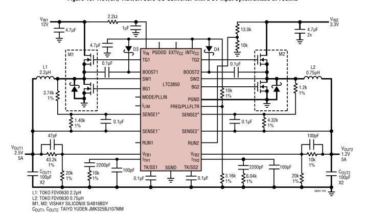
Figure 20. 2.5V/5A, 1.2V/5A Core-I/O Converter with Dual Inputs
