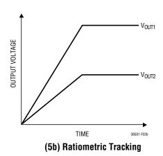
Figure 5. Two Different Modes of Output Voltage Tracking
