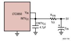
Figure 8. Setup for a 5V Input
