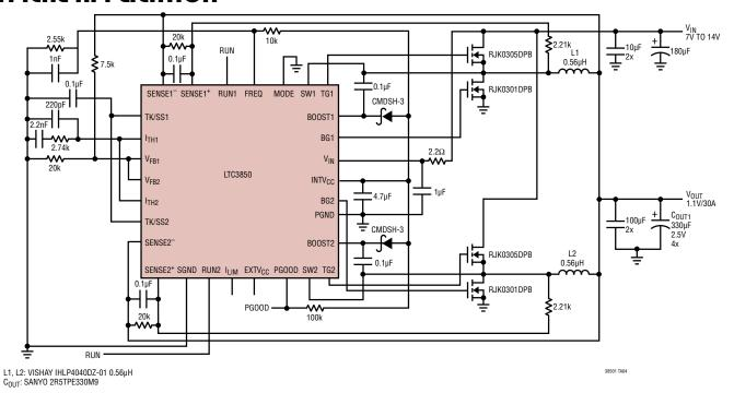
FOR SINGLE OUTPUT, DUAL PHASE OPERATION, TIE THE FOLLOWING PINS TOGETHER: VFB1 TO VFB1 TK/SS1 TO TK/SS2 ITH1 TO ITH2 RUN1 TO RUN2
