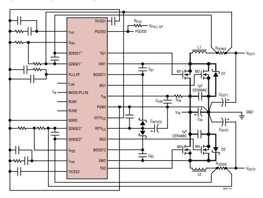
Figure 13. Recommended Printed Circuit Layout Diagram
