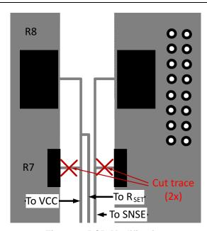
Figure 2. PCB Modification
