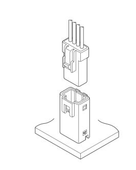
This JWPF connector can be used for the place of which especially waterproof is required.
