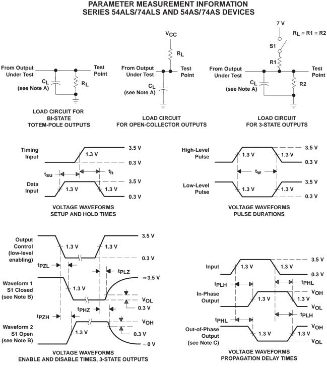
NOTES: A. C<sub>1</sub> includes probe and jig capacitance.
