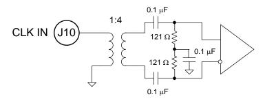
Figure 5. ADS4449 Clock Input Circuit
