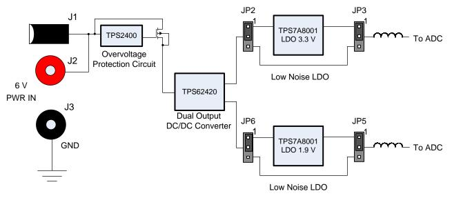
Figure 2. Simplified ADS4449 EVM Power Supply
