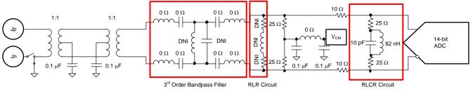
Figure 4. ADS4449 ADC Input Circuit
