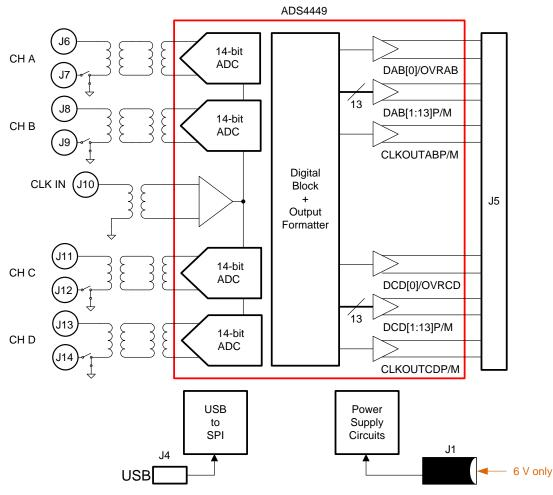
Figure 1. Simplified ADS4449 EVM Block Diagram
