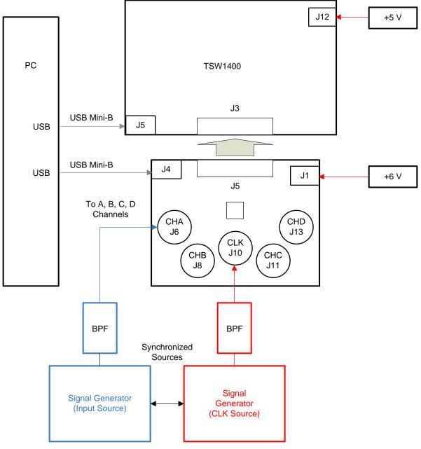
Figure 8. ADS4449 and TSW1400 Test Setup Block Diagram
