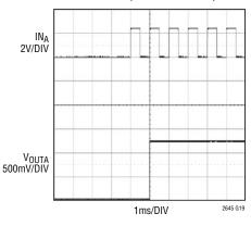
Exiting Idle Mode Full-Scale to Mid-Scale (IDLSEL = GND)
