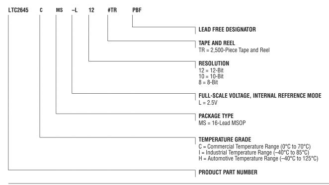
Contact the factory for parts specified with wider operating temperature ranges. \*The temperature grade is identified by a label on the shipping container.
