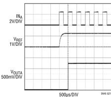
Power-On-Reset to Idle Mode Full-Scale (IDLSEL = GND)
