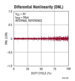
LTC2645-8 (Internal Reference,  $V_{FS} = 2.5V$ )
