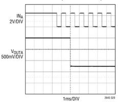
Exiting Idle Mode Power-Down (1 Channel) to Mid-Scale (IDLSEL = V<sub>CC</sub>)
