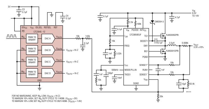
Figure 4. Voltage Margining Application with LTC3850 (3.3V ±10%)
