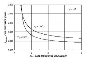
Figure 4. On-Resistance Variation with Gate-to-Source Voltage.
