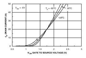
Figure 5. Transfer Characteristics.
