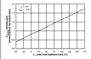
Figure 3. On-Resistance Variation with Temperature.
