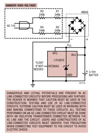
Figure 5. 4.2V AC Line Charging, UL Leakage Okay
