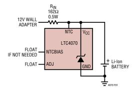
Figure 1. Single-Cell Battery Charger
