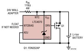
Figure 2. Single-Cell Charger with Boosted Drive
