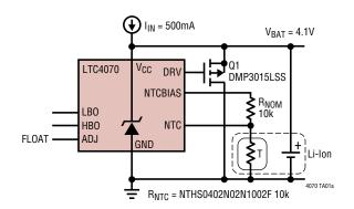
Figure 8. Replace Three NiMH with Lithium
