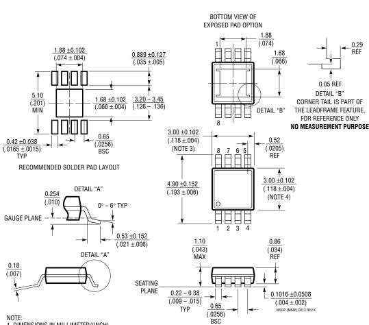
**MS8E** Package 8-Lead Plastic MSOP, Exposed Die Pad (Reference LTC DWG # 05-08-1662 Rev K)
