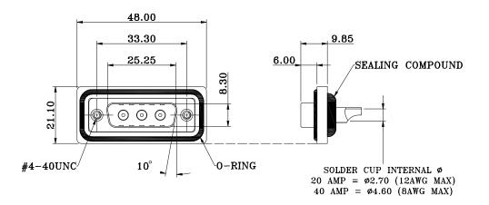
NOTE: **MATERIAL** HOUSING PBT UL94V-0, BLACK FLANGE PBT UL94V-0, BLACK CONTACT BRASS, PLATING P/N KEY BELOW SHELL STEEL, NICKEL O-RING SILICONE **EPOXY** SEALING COMPOUND HARDWARE BRASS; NICKEL PLATED ELECTRICAL POWER CONTACT RATED CURRENT P/N KEY BELOW VOLTAGE 1000 VAC 1 MIN INSULATOR RESISTANCE 5 G0hms MIN. POWER CONTACT RESISTANCE 1.0 m0hms MAX. WATER PROOF **IP67**
