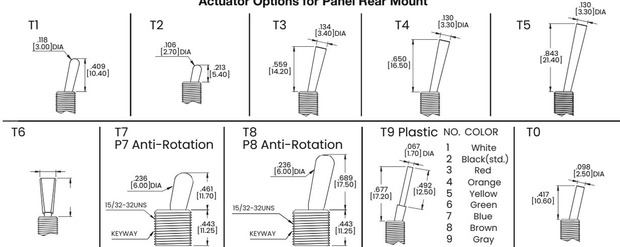
\* T6 actuator is available with B1, B2, B5, B6, BA, BB & BE bushing. Actuator length shown for T1-T5, T9 and T10 is with B1 bushing. T7, T7, P8 does not require a bushing code.
