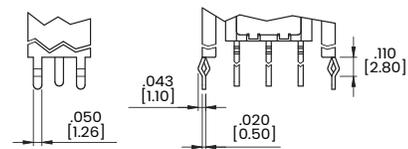
\* PC Mounting for M61,M71,VS21,VS31,VS41,VS51 refer to M6,M7,VS2,VS3,VS4,VS5 respectively.
