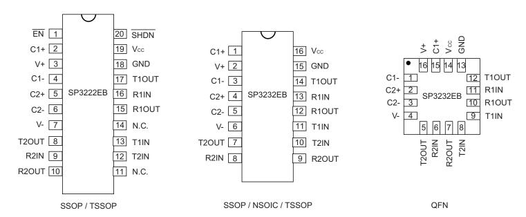
Figure 7: Pinout Configurations for the SP3222EB and SP3232EB
