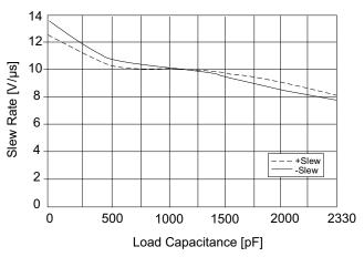
Figure 3: Slew Rate vs. Load Capacitance
