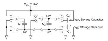
Figure 13: Charge Pump — Phase 1
