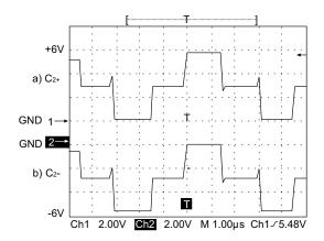
Figure 15: Charge Pump Waveforms
