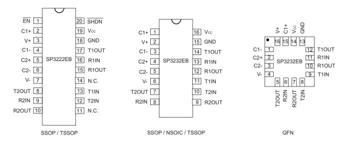
Figure 1: SP3222EB and SP3232EB Pinouts
