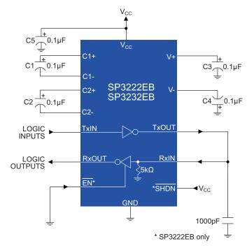
Figure 10: SP3222EB / SP3232EB Driver Loopback Test Circuit
