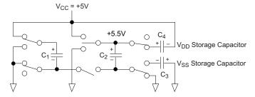
Figure 17: Charge Pump — Phase 4
