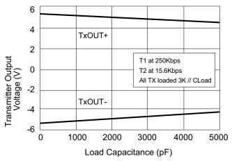
Figure 2: Transmitter Output Voltage vs. Load Capacitance
