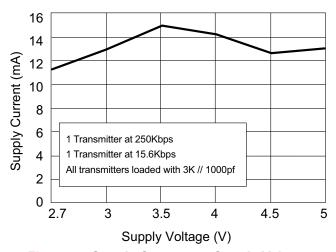
Figure 5: Supply Current vs. Supply Voltage
