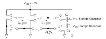
Figure 14: Charge Pump — Phase 2
