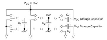
Figure 16: Charge Pump — Phase 3
