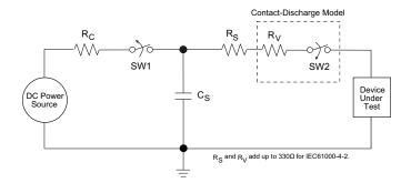
Figure 19: ESD Test Circuit for IEC61000-4-2
