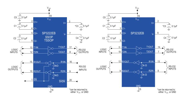
Figure 8: SP3222EB Typical Operating Circuit
