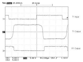
Figure 11: Loopback Test Results at 120kbps
