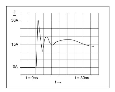
Figure 20: ESD Test Waveform for IEC61000-4-2
