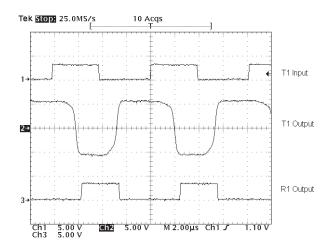
Figure 12: Loopback Test Results at 250kbps
