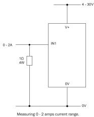
$\label{eq:continuous} \begin{tabular}{ll} \mbox{Measuring 0 - 2 amps current range.} \\ \mbox{Use a 1 } \Omega \mbox{ resistor, with a 4W rating.} \\ \mbox{Setup scaling in software: 0V = 0.00 and 2V = 2.00} \end{tabular}$
