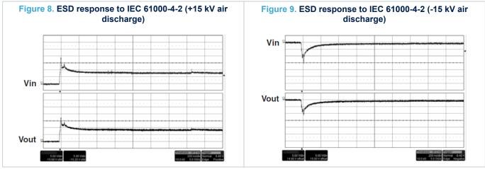
*Note: Important*: A good precaution to take is to put the protection device as close as possible to the disturbance source (generally the connector).
