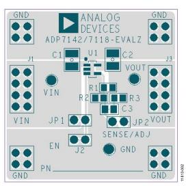
Figure 2. ADP7118/ADP7142 TSOT Evaluation Board
