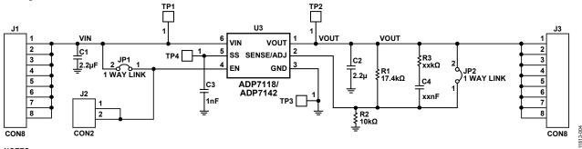
NOTES 1. THE VALUES OF R3 AND C4 DEPEND ON THE LOW FREQUENCY ZERO OF THE NOISE REDUCTION NETWORK. SEE DATA SHEET FOR DESIGN DETAILS. Figure 4. LFCSP Evaluation Board Schematic
