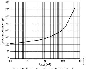
Figure 16. Ground Current vs. Load Current (ILOAD)
