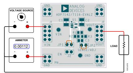
Figure 15. Ground Current Measurement, TSOT
