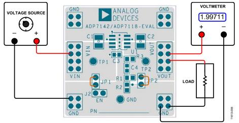
Figure 8. Output Voltage Measurement, SOIC
