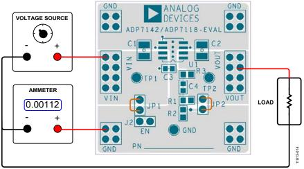
Figure 14. Ground Current Measurement, SOIC
