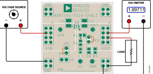
Figure 7. Output Voltage Measurement, LFCSP
