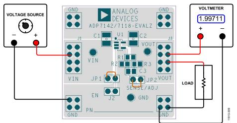
Figure 9. Output Voltage Measurement, TSOT
