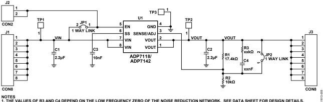
NOTES 1. THE VALUES OF R3 AND C4 DEPEND ON THE LOW FREQUENCY ZERO OF THE NOISE REDUCTION NETWORK. SEE DATA SHEET FOR DESIGN DETAILS. Figure 5. SOIC Evaluation Board Schematic
