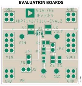
Figure 1. ADP7118/ADP7142 LFCSP Evaluation Board
