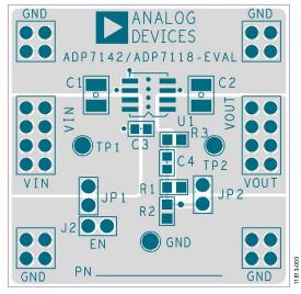
Figure 3. ADP7118/ADP7142 SOIC Evaluation Board
