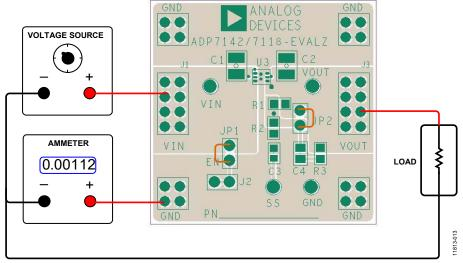
Figure 13. Ground Current Measurement, LFCSP
