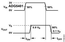
Figure 26. Switching Times, ton and toff
