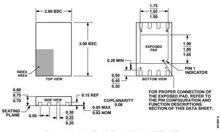
Figure 30. 8-Lead Lead Frame Chip Scale Package [LFCSP\_WD] 2 mm × 3 mm Body, Very Very Thin, Dual Lead (CP-8-4) Dimensions shown in millimeters
