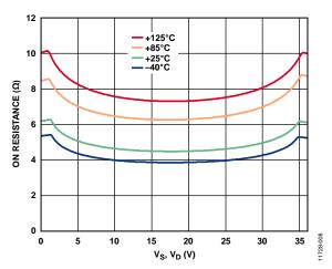
Figure 9. On Resistance as a Function of  $V_5$  ( $V_0$ ) for Different Temperatures, 36 V Single Supply
