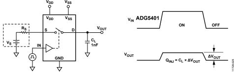
Figure 27. Charge Injection
