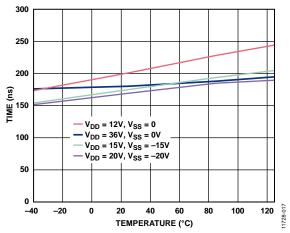
Figure 18. ttransition Times vs. Temperature
