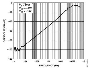
Figure 14. Off Isolation vs. Frequency
