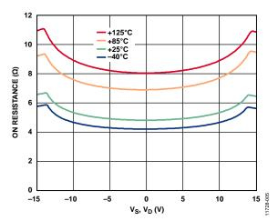
Figure 6. On Resistance as a Function of  $V_S(V_D)$  for Different Temperatures,  $\pm 15 \text{ V Dual Supply}$
