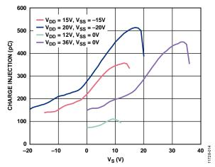
Figure 15. Charge Injection vs. Source Voltage (V<sub>S</sub>)
