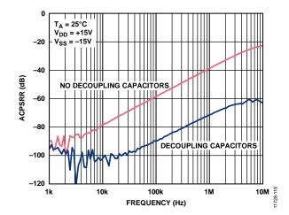
Figure 19. ACPSRR vs. Frequency
