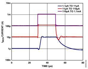
Figure 28. I<sub>MON</sub> Pulse Response vs. I<sub>NUM</sub>
