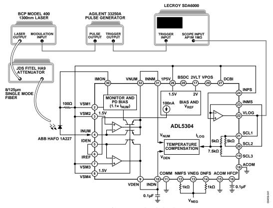
Figure 41. Setup for Measuring Photodiode Pulse Response
