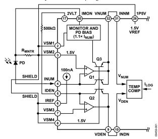
Figure 52. Intercept Shifted One Decade Right via External Resistor, Reference Current I<sub>DEN</sub> = 1 μA
