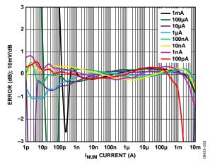
Figure 8. Law Conformance Error vs. I<sub>NUM</sub> for Multiple Values of I<sub>DEN</sub> (Decade Steps from 100 pA to 1 mA)
