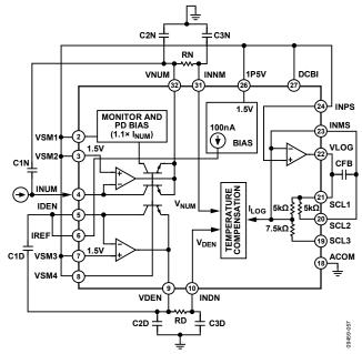
Figure 48. Possible External Filtering Locations
