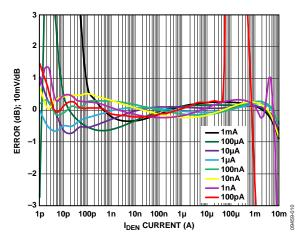
Figure 12. Law Conformance Error vs. I<sub>DEN</sub> for Multiple Values of I<sub>NUM</sub> (Decade Steps from 100 pA to 1 mA)
