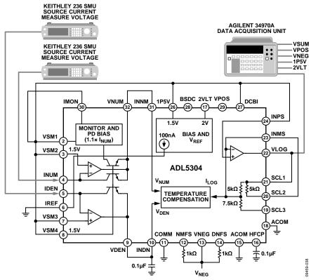
Figure 38. Setup for Measuring Logarithmic/Slope/Offset Conformance
