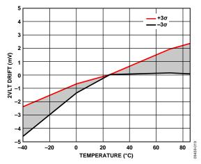
Figure 19. 2VLT Drift vs. Temperature
