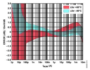
Figure 13. Law Conformance Error Distribution vs.  $I_{NUM}$  for  $-40^{\circ}$ C and  $+85^{\circ}$ C (3  $\sigma$  Either Side of Mean)
