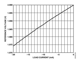
Figure 20. 2VLT vs. I<sub>LOAD</sub> (Positive Current Defined into 2VLT Pin)
