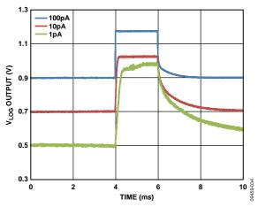
Figure 57. Increased Time Scale to Show Measurements Down to I<sub>NUM</sub> Approximately 1 pA (Approximately 1.25 pW; –89.03 dBm)
