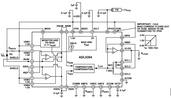
Figure 55. Basic Connections for Single-Supply Operation
