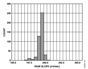
Figure 34. Distribution of Logarithmic Slope (Nominally 200 mV/dec)
