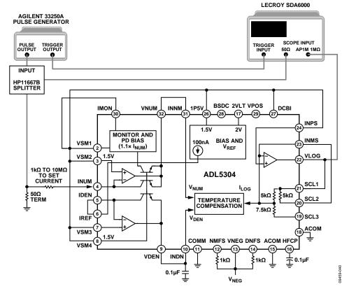
Figure 40. Setup for Measuring Pulse Settling
