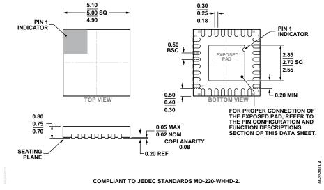
Figure 61. 32-Lead Lead Frame Chip Scale Package [LFCSP] 5 mm × 5 mm Body and 0.75 mm Package Height (CP-32-21) Dimensions shown in millimeters
