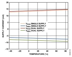
Figure 37. Supply Current vs. Temperature ( $|V_{POS}|$ ,  $|V_{VNEG}|$ )
