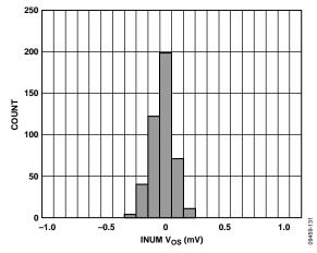
Figure 31. (V<sub>NUM</sub> – V<sub>SUM</sub>) Histogram at 25°C
