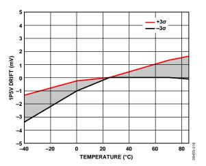
Figure 16. 1P5V Drift vs. Temperature
