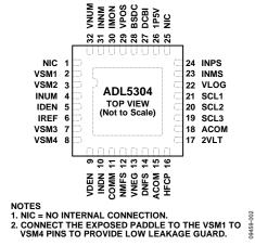
Figure 2. 32-Lead LFCSP Pin Configuration
