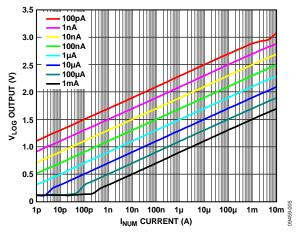
Figure 5. V<sub>LOG</sub> vs. I<sub>NUM</sub> for Multiple Values of I<sub>DEN</sub> (Decade Steps from 100 pA to 1 mA)
