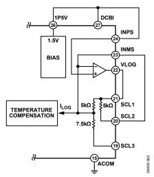
Figure 51. Buffer Amplifier in Default Configuration
