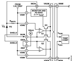
Figure 53. Simple Slope Inversion Method
