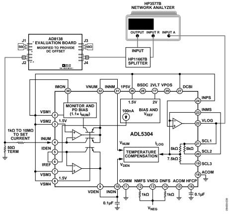
Figure 39. Setup for Measuring Bandwidth
