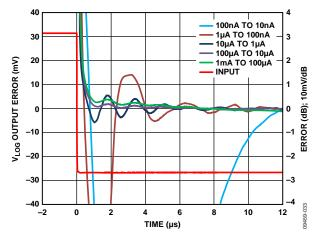
Figure 26. Normalized Falling Edge Settling of I<sub>NUM</sub> to Within 1 dB (Error = 10 mV/dB)
