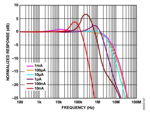
Figure 24. Small Signal AC Response from I<sub>DEN</sub> to V<sub>LOG</sub> for I<sub>DEN</sub> in Decade Steps from 10 nA to 1 mA; I<sub>NUM</sub> = 100 nA
