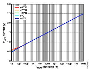
Figure 3. V<sub>LOG</sub> vs. I<sub>NUM</sub> for Multiple Temperatures
