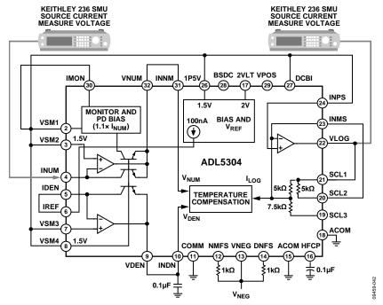
Figure 42. Setup for Measuring Output
