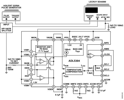
Figure 43. Setup for Measuring IMON Pulse Response
