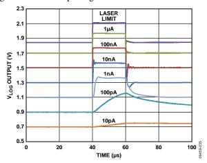
Figure 56. Photodiode Response for Input Currents of Approximately 10 pA to >1 μA Where Laser Limit Encountered
