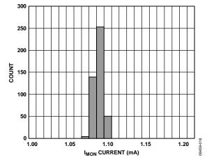
Figure 18.  $I_{MON}$  Histogram at  $I_{NUM} = 1$  mA
