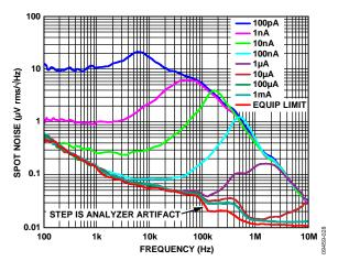
Figure 22. Spot Noise Spectral Density at VLOG vs. Frequency for I<sub>NUM</sub> in Decade Steps from 1 nA to 1 mA (Noise at lower frequencies, where NSD is flat, is limited by resistance used to generate dc I<sub>NUM</sub> current. See the Noise vs. Current section for further explanation.)
