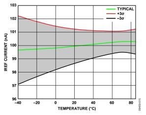
Figure 15. IREF Current vs. Temperature
