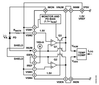
Figure 45. Simplified Front-End Schematic
