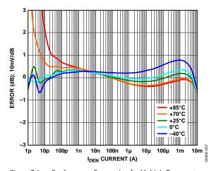
Figure 7. Law Conformance Error vs.  $I_{DEN}$  for Multiple Temperatures;  $I_{NUM}=100$  nA; Normalized to 25°C
