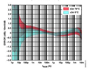
Figure 11. Law Conformance Error Distribution vs.  $I_{NUM}$  for 0°C and 70°C (3  $\sigma$  Either Side of Mean)
