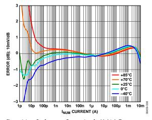
Figure 6. Law Conformance Error vs.  $I_{NUM}$  for Multiple Temperatures; Normalized to 25  $^{\circ}$ C
