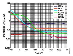
Figure 25. Spot Noise Spectral Density at VLOG vs. I<sub>NUM</sub> in Decade Frequency Steps from 100 Hz to 10 MHz
