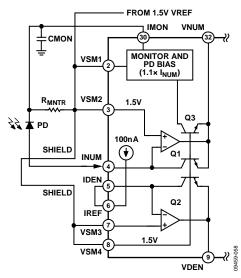
Figure 49. Adaptive Photodiode Bias
