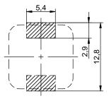
no sensitive traces underneath the component
