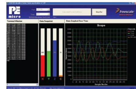
AccelerometerDemo running on MC9S08QE32 in data averaging mode. Bar graph 'C' highlights the bus cycles required to average the last 16 readings of the 3 axes. The value in the 4th column in the terminal window is the number of bus cycles in hex.
