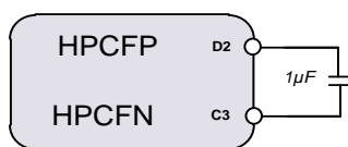
Figure 39: Charge pump flying capacitor
