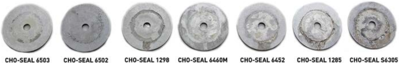
Figure 2-2: Picture of Corrosion Coupon After 504 salt spray/salt fog
