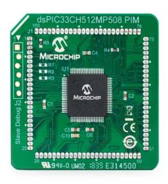
dsPIC33CH512MP508 GP Plug-In Module (Part # MA330046)
