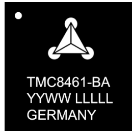
Figure 52: TMC8461-BA device marking
