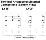
Note: The figures and dimensions depicted here are for the LY1F. The LY2F is also conforms to these measurements.
