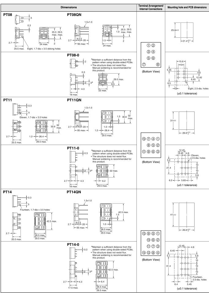
Note: Use a panel with a thickness of 1 to 2 mm when mounting a Socket on it.
