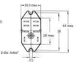
Two, 3.5-dia, holes or two M3 screw holes
