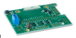
Also RS-232 signals at display are 3.3V level; this application board provides a level shifter for ±12V level (for pc).
