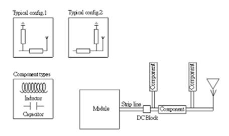
Matching should be considered using a Pi network where 1, 2 or 3 components could be used. This shall be matched to the transmission line and the ground plane in the design.
