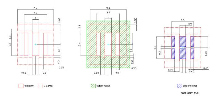
For superior solder joint connectivity results we recommend soldering under standard nitrogen atmosphere. Further information can be found in our Application Note: "Handling and Processing Details for Ceramic LEDs". Package not suitable for any kind of wet cleaning or ultrasonic cleaning.
