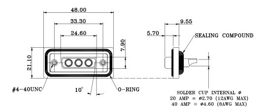
NOTE: **MATERIAL** HOUSING PBT UL94V-0, BLACK FLANGE PBT UL94V-0, BLACK CONTACT BRASS, PLATING P/N KEY BELOW SHELL STEEL, NICKEL O-RING SILICONE **EPOXY** SEALING COMPOUND HARDWARE BRASS; NICKEL PLATED ELECTRICAL POWER CONTACT RATED CURRENT P/N KEY BELOW VOLTAGE 1000 VAC 1 MIN INSULATOR RESISTANCE 5 G0hms MIN. POWER CONTACT RESISTANCE 1.0 m0hms MAX. WATER PROOF **IP67** ENVIRONMENT
