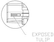
USE ABOVE FRONT FACE DIMENSIONS FOR PCB LAYOUT DESIGN. Ø0.8mm HOLE SIZE IS RECOMMENDED.
