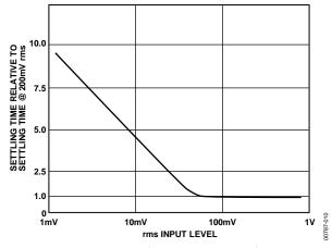
Figure 14. Settling Time vs. Input Level
