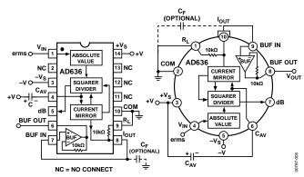
Figure 9. Standard RMS Connection
