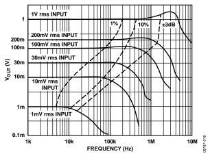
Figure 5. AD636 Frequency Response
