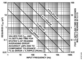
Figure 13. Error/Settling Time Graph for Use with the Standard RMS Connection
