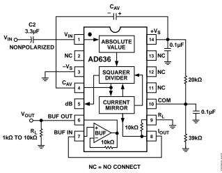
Figure 11. Single-Supply Connection (See Text)
