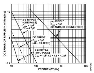
Figure 16. Performance Features of Various Filter Types
