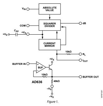
The AD636 is available in two accuracy grades. The total error of the J-version is typically less than  $\pm 0.5$  mV  $\pm 1.0\%$  of reading, while the total error of the AD636K is less than  $\pm 0.2$  mV to  $\pm 0.5\%$  of reading. Both versions are temperature rated for operation between 0°C and 70°C and available in 14-lead SBDIP and 10-lead TO-100 metal can.
