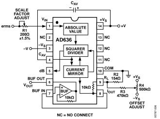
Figure 10. Optional External Gain and Output Offset Trims
