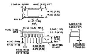
CONTROLLING DIMENSIONS ARE IN INCHES; MILLIMETER DIMENSIONS (IN PARENTHESES) ARE ROUNDED-OFF INCH EQUIVALENTS FOR REFERENCE ONLY AND ARE NOT APPROPRIATE FOR USE IN DESIGN.
