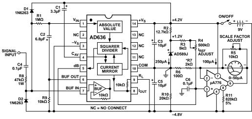
ALL RESISTORS 1/4W 1% METAL FILM UNLESS OTHERWISE STATED EXCEPT \*WHICH IS  $2k\Omega$  +3500ppm 1% TC RESISTOR.
