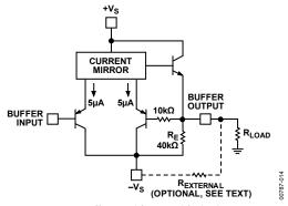
Figure 8. Buffer Amplifier Simplified Schematic
