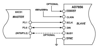
Figure 37. 8XC51/PIC16C42 Interface
