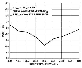
Figure 20. PSRR vs. Frequency
