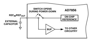
Figure 23. On-Chip Reference During Power-Down
