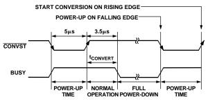
Figure 22. Power-Up Timing When Using CONVST Pin
