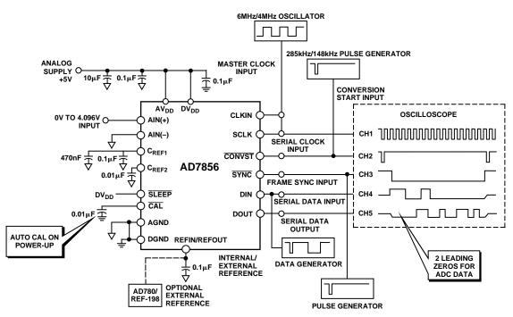
Figure 10. Typical Circuit
