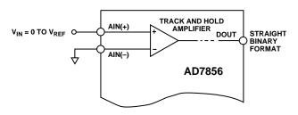
Figure 14. 0 to V<sub>REF</sub> Input Configuration
