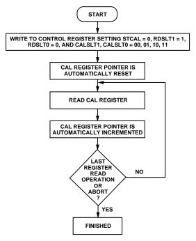
*Figure 9. Flowchart for Reading from the Calibration Registers*
