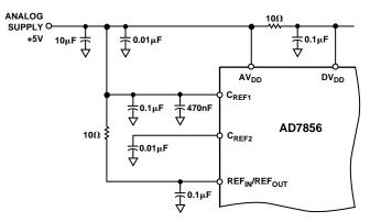
Figure 17. Relevant Connections When Using  $AV_{\text{DD}}$  as the Reference
