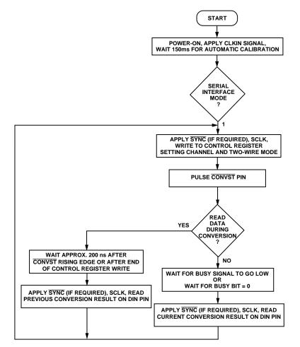
Figure 34. Flowchart for Setting Up, Reading and Writing in Interface Mode 1
