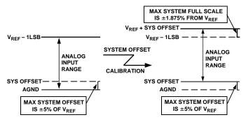
Figure 26. System Offset Calibration
