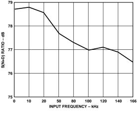
Figure 19. SNR vs. Frequency
