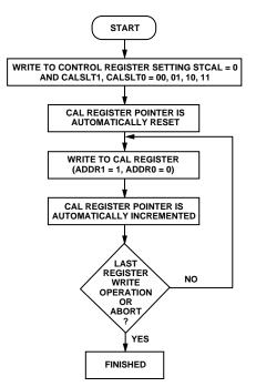
*Figure 8. Flowchart for Writing to the Calibration Registers*
