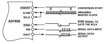
Figure 36. Simplified Interface Diagram
