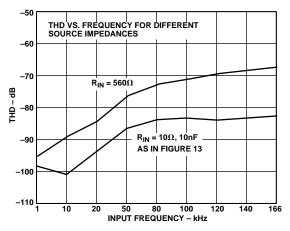
Figure 12. THD vs. Analog Input Frequency
