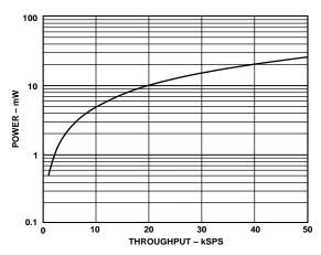
Figure 24. Power vs. Throughput Rate (6 MHz CLK)
