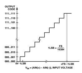
Figure 15. Transfer Characteristic
