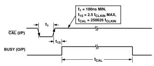
Figure 25. Timing Diagram for Full-Self Calibration
