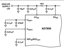
Figure 16. Relevant Connections When Using Internal Reference
