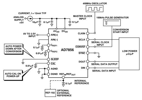
Figure 21. Typical Low Power Circuit
