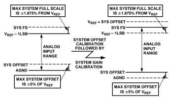
Figure 28. System (Gain + Offset) Calibration
