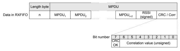
Figure 43: Data in RXFIFO when MDMCTRLOL.AUTOCRC is set
