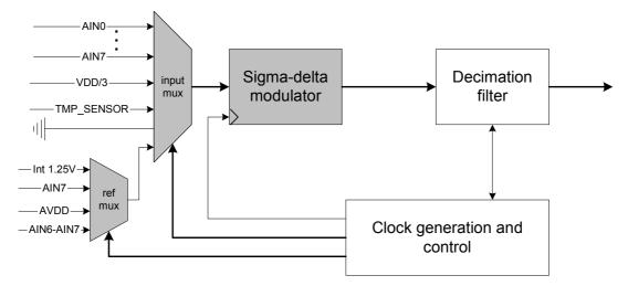
Figure 26: ADC block diagram.
