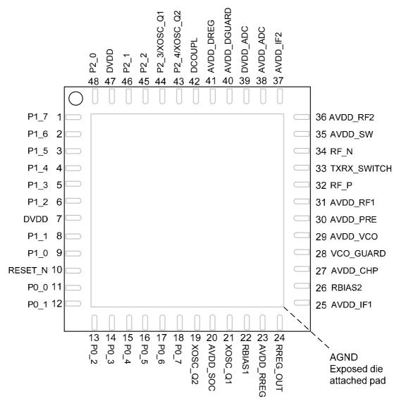
Figure 4: Pinout top view
