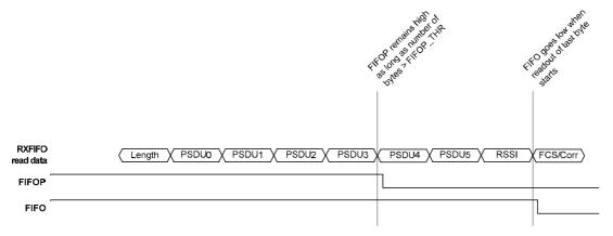
Figure 36: Example of status activity when reading RXFIFO.
