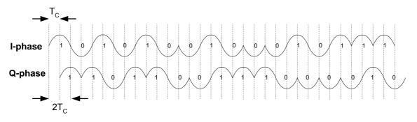
Figure 34: I / Q Phases when transmitting a zero-symbol chip sequence,  $T_c = 0.5 \mu s$
