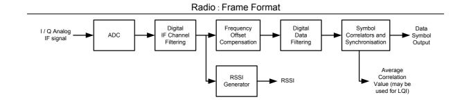
Figure 38: Demodulator Simplified Block Diagram
