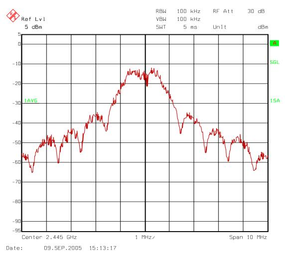
Figure 49: Modulated spectrum plot
