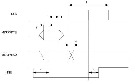
Figure 2: SPI AC Characteristics
