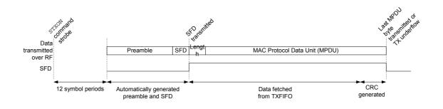
Figure 37: SFD status activity example during transmit
