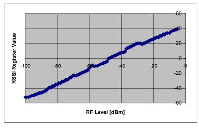
Figure 47: Typical RSSI value vs. input power
