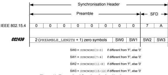
Figure 40: Transmitted Synchronization Header
