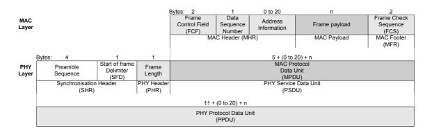
Figure 39: Schematic view of the IEEE 802.15.4 Frame Format [1]
