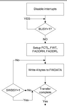
Figure 16: Performing CPU Flash write
