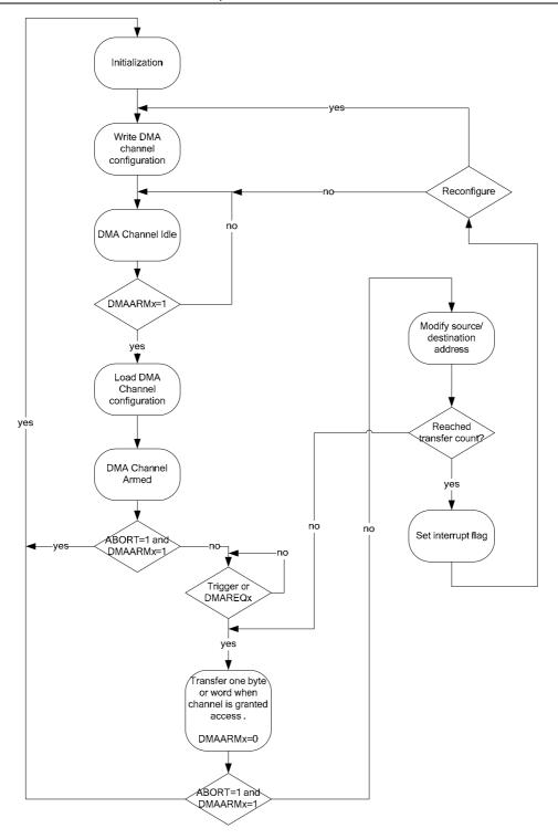
Figure 18: DMA Operation
