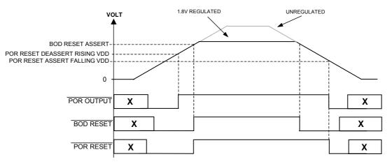
Figure 13 : Power On Reset and Brown Out Detector Operation
