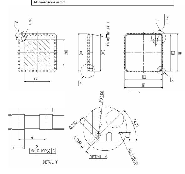
Figure 51: Package dimensions drawing
