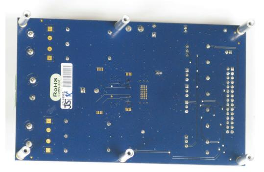
Figure 2. The TI DRV8412EVM Motor Drive Evaluation Board – Bottom View
