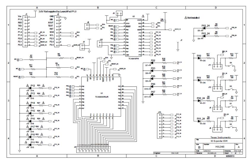
Figure 5. IO Expander EVM Schematic
