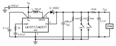
L = 415-0930 (AIE) D = any manufacturer  $C_{OUT}$  = Sprague Type 673D Electrolytic 680  $\mu$ F, 20V
