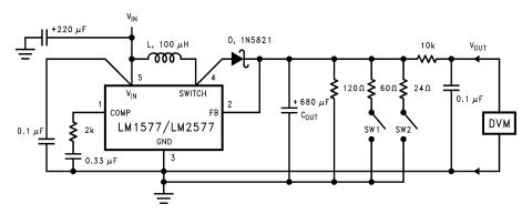
L = 415-0930 (AIE) D = any manufacturer C<sub>OUT</sub> = Sprague Type 673D
