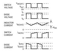
Figure 12. Step-Up Regulator Waveforms
