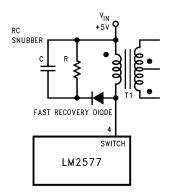
Figure 23. Snubber Circuit
