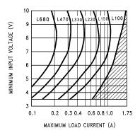
Figure 13. LM2577-12 Inductor Selection Guide
