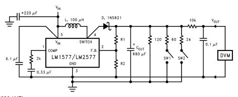
L = 415-0930 (AIE) D = any manufacturer  $C_{OUT} = \text{Sprague Type 673D}$   $Electrolytic 680 \ \mu\text{F, 20V}$   $R1 = 48.7k \text{ in series with } 511\Omega \text{ (1%)}$
