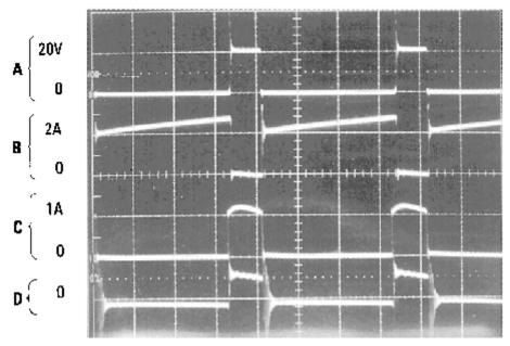
A: Switch pin voltage, 20 V/div
