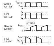
Figure 20. Flyback Regulator Waveforms
