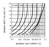
Figure 14. LM2577-15 Inductor Selection Guide
