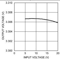
Figure 11. Line Regulation - L1 = 10  $\mu H$  V<sub>OUT</sub> = 3.3 V, I<sub>OUT</sub> = 500 mA
