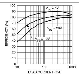
Figure 20. Efficiency vs Load Current - L1 = 10  $\mu$ H V<sub>OUT</sub> = 3.3 V
