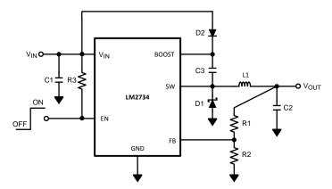
Figure 27. LM2734Y (550 kHz)  $V_{\text{BOOST}}$  Derived from  $V_{\text{IN}}$  5 V to 1.5 V / 1-A Schematic
