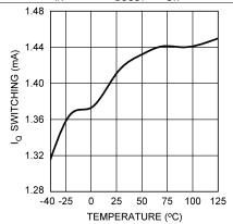
Figure 7.  $I_Q$  Switching vs Temperature
