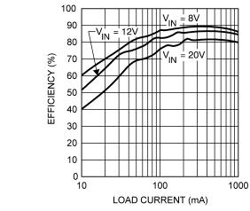
Figure 17. Efficiency vs Load Current - L1 = 4.7  $\mu$ H V<sub>OUT</sub> = 5 V
