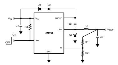
Figure 30. LM2734Y (550 kHz) V<sub>BOOST</sub> Derived from Series Zener Diode (V<sub>IN</sub>) 15 V to 1.5 V / 1-A Schematic
