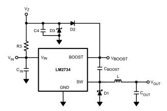
Figure 15. Boost Voltage Supplied from the Shunt Zener on VIN
