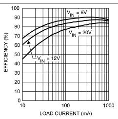
Figure 18. Efficiency vs Load Current - L1 = 10  $\mu$ H V<sub>OUT</sub> = 5 V
