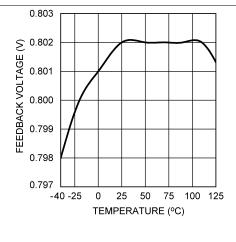
Figure 5. V<sub>FB</sub> vs Temperature
