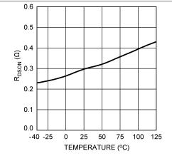
Figure 6. R<sub>DSON</sub> vs Temperature
