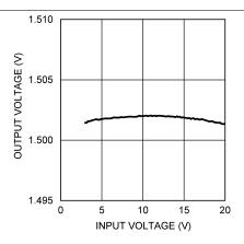
Figure 9. Line Regulation - L1 = 10  $\mu H$   $V_{OUT}$  = 1.5 V,  $I_{OUT}$  = 500 mA
