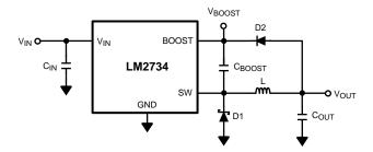
Figure 13. V<sub>OUT</sub> Charges C<sub>BOOST</sub>
