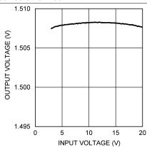
Figure 8. Line Regulation - L1 = 4.7  $\mu$ H V<sub>OUT</sub> = 1.5 V, I<sub>OUT</sub> = 500 mA
