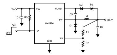
Figure 26. LM2734X (1.6 MHz) V<sub>BOOST</sub> Derived from Series Zener Diode (V<sub>OUT</sub>) 15 V to 9 V /1-A Schematic
