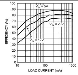
Figure 19. Efficiency vs Load Current - L1 = 4.7  $\mu$ H V<sub>OUT</sub> = 3.3 V
