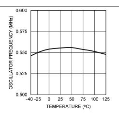
Figure 1. Oscillator Frequency vs Temperature - L1 = 4.7 μH
