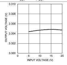
Figure 10. Line Regulation - L1 = 4.7  $\mu$ H V<sub>OUT</sub> = 3.3 V, I<sub>OUT</sub> = 500 mA
