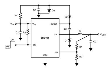
Figure 24. LM2734X (1.6 MHz) V<sub>BOOST</sub> Derived from V<sub>SHUNT</sub> 18 V to 1.5 V /1-A Schematic
