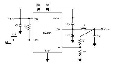
Figure 25. LM2734X (1.6 MHz) V<sub>BOOST</sub> Derived from Series Zener Diode (V<sub>IN</sub>) 15 V to 1.5 V / 1-A Schematic
