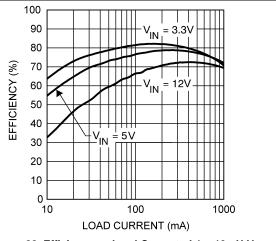
Figure 22. Efficiency vs Load Current - L1 = 10  $\mu$ H V<sub>OUT</sub> = 1.5 V
