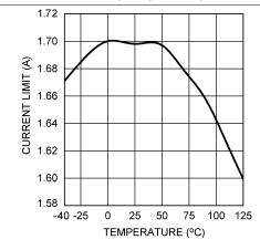
Figure 3. Current Limit vs Temperature
