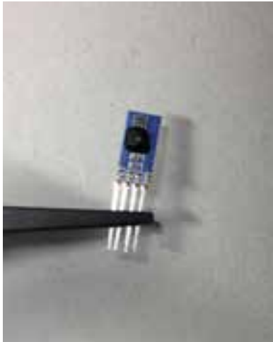
Sensor held with plastic tweezers on the wires only
