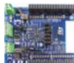
STEVAL-IOM001V1 IO-Link master evaluation board based on L6360 equipped with ST morpho connectors for STM32 Nucleo
