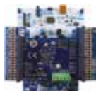
P-NUCLEO-IOD01A1 STM32 Nucleo pack for IO-Link device fully compatible with IO-Link v1.1 (PHY and stack)
