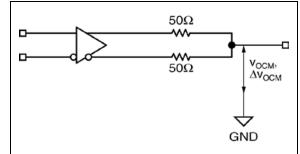
FIGURE 7-2: LVDS Common Mode Measurement.
