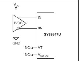
FIGURE 6-5: LVDS Interface (DC-Coupled).
