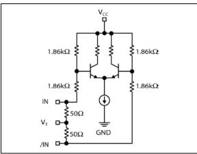
*FIGURE 5-8:* Simplified Differential Input Stage.
