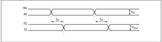
FIGURE 5-3: Propagation Delay.
