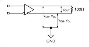
FIGURE 7-1: LVDS Differential Measurement.
