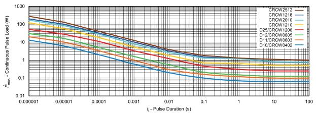
Maximum pulse load, continuous pulses; applicable if  $\overline{P} \leq P$  ( $\mathcal{G}_{amb}$ ) and  $\hat{U} = \hat{U}_{max}$ ; for permissible resistance change equivalent to 8000 h operation
