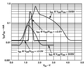
TPC 5. Supply Current vs. Logic Input Voltage
