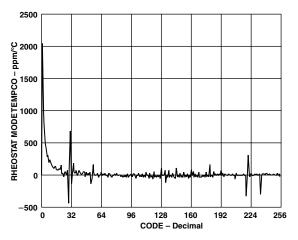
TPC 21.  $\Delta R_{WB}/\Delta T$  Rheostat Mode Temperature Coefficient
