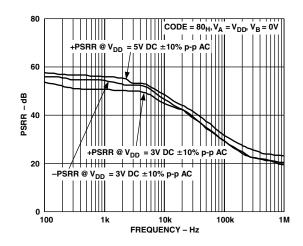
TPC 11. Power Supply Rejection Ratio vs. Frequency
