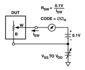
Figure 17. Incremental ON Resistance Test Circuit
