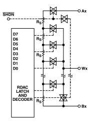
Figure 8. Equivalent RDAC Circuit
