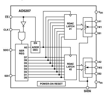
Figure 2. Block Diagram
