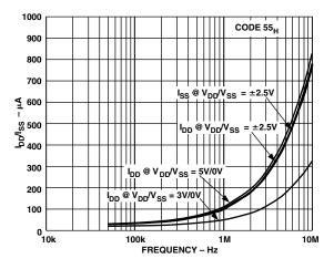
TPC 10. 10  $k\Omega$  Supply Current vs. Clock Frequency
