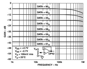
TPC 12. 10 k $\Omega$  Gain vs. Frequency vs. Code
