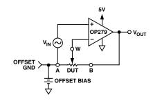
Figure 15. Noninverting Gain Test Circuit
