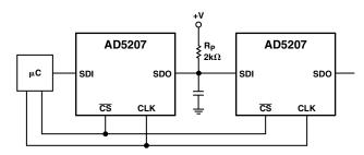
Figure 3. Daisy-Chain Configuration Using SDO
