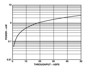
Figure 2. Power vs. Throughput
