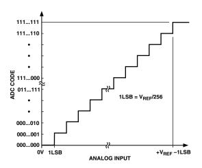
Figure 11. Transfer Characteristic
