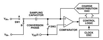
Figure 5. ADC Conversion Phase
