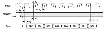
Figure 16. Serial Interface Timing
