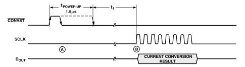
Figure 15. Mode 2 Operation Timing
