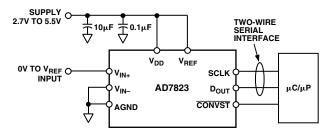
Figure 6. Typical Connection Diagram
