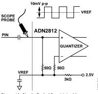
Figure 13. Single-Ended Sensitivity Measurement
