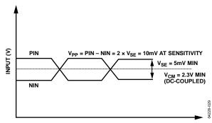
Figure 29. Minimum Allowed DC-Coupled Input Levels
