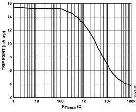
Figure 5. LOS Comparator Trip Point Programming
