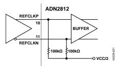
Figure 21. Differential REFCLK Configuration
