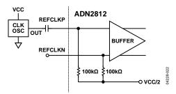
Figure 22. Single-Ended REFCLK Configuration
