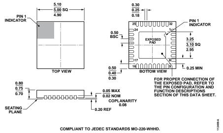
Figure 31. 32-Lead Lead Frame Chip Scale Package [LFCSP\_WQ] 5 mm × 5 mm Body, Very Thin Quad (CP-32-7) Dimensions shown in millimeters
