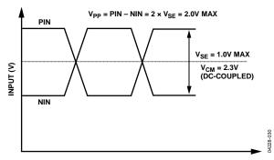
Figure 30. Maximum Allowed DC-Coupled Input Levels
