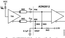
Figure 26. ADN2812 AC-Coupled Input Configuration
