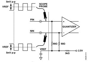
Figure 14. Differential Sensitivity Measurement
