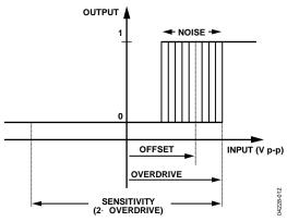
Figure 12. Input Sensitivity and Input Overdrive
