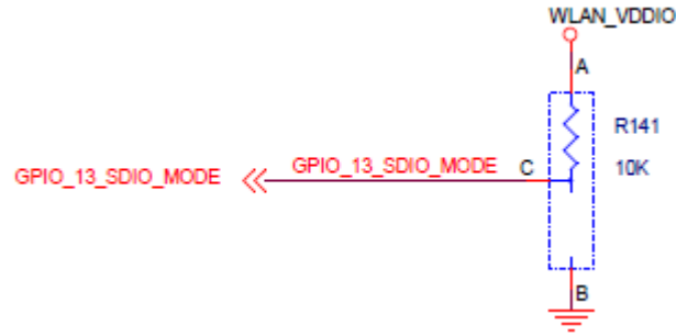
Figure 4-8. GPIO_13_SDIO_MODE Strapping Option
