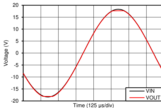
Figure 7-1. Output Waveform Devoid of Phase Reversal During an Input Overdrive Condition
