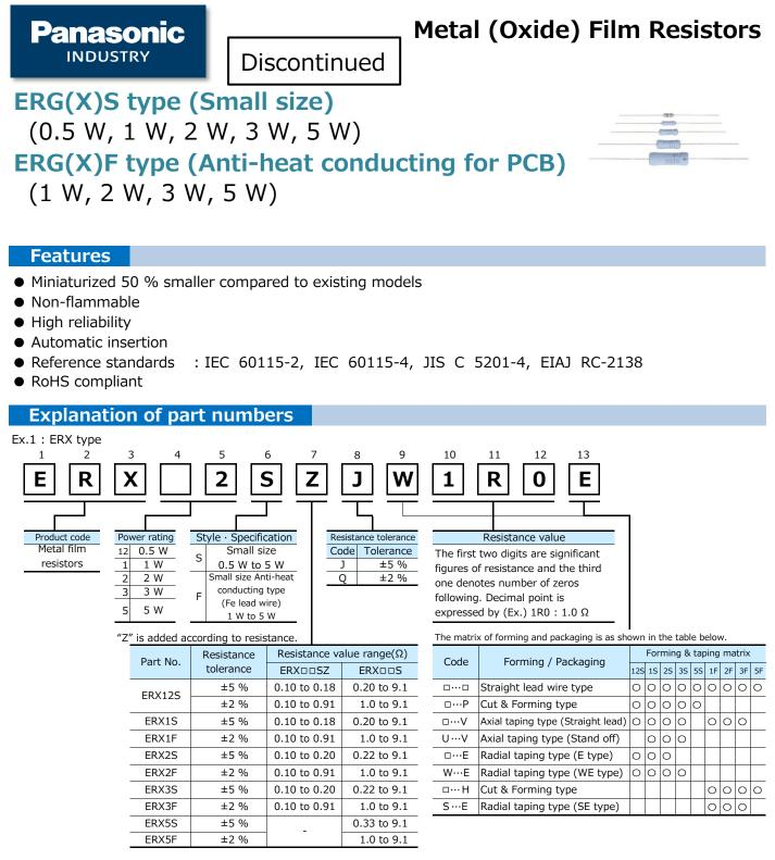
The above example 1 shows a small metal film resistor, 2 W power rating, resistance value of 1.0  $\Omega$ , tolerance ±5 %, and package of radial taping.
