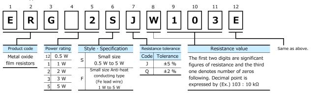
The above example 2 shows a small metal oxide film resistor, 2 W power rating, resistance value of 10 k $\Omega$ , tolerance ±5 %, and package of radial taping.
