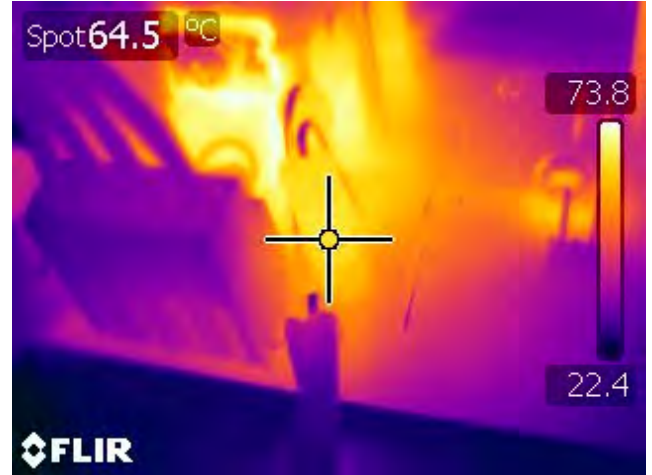
Figure 58 – Current Sense Resistor (R53), 90 VAC Input, 100% Load, Room Temperature.
