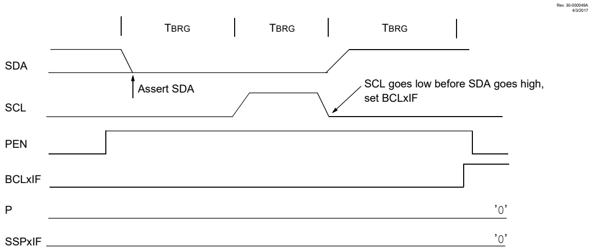
Figure 25-40. Bus Collision During a Stop Condition (Case 2)
