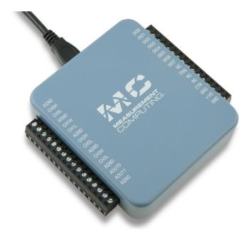
USB-230 Series devices provide eight SE/four DIFF analog inputs, two simultaneously-updating analog outputs, 8 digital I/O, and one counter input.
