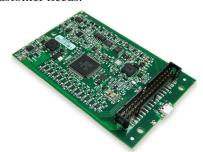
The OEM versions have the same specifications as the standard devices, but come in a board-only form factor with a header connector instead of screw terminals.
