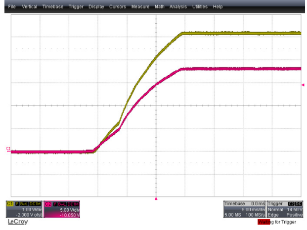
Figure 32 – Start-up Profile, 265 VAC, Full CC Load. Upper: V_{OUT} , 5 V, 1 V / div. Lower: V_{OUT} , 18 V, 5 V, 5 ms / div.
