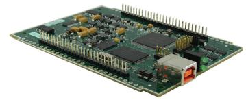
The OEM versions have the same specifications as the standard devices, but come in a board-only form factor with header connectors instead of screw terminals.
